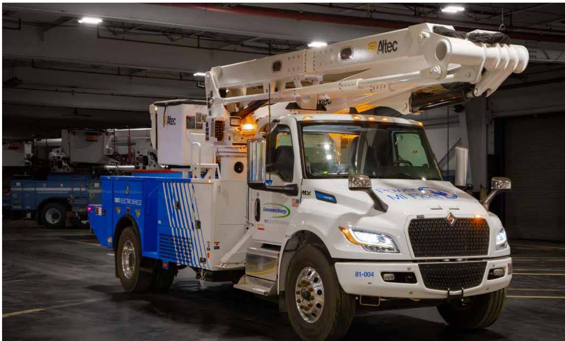
CONSUMERS ENERGY'S ALL-ELECTRIC BUCKET TRUCK (COURTESY OF CONSUMERS ENERGY)
